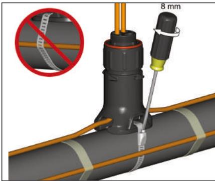
4. Temporarily mount expediter to pipe using pipe band. Do not band over cable.
