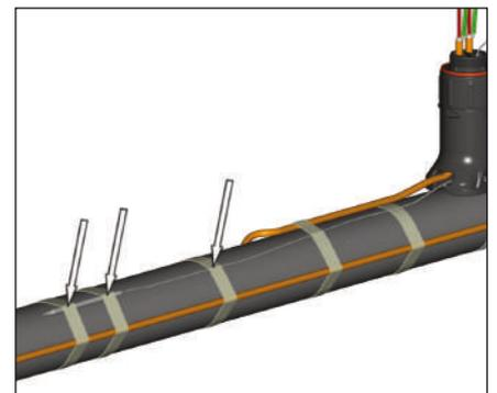
12. Fix thermostat bulb and capillary tube to pipe.
