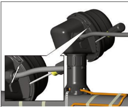
**19.** Lid latch mechanism fully engaged. To remove lid, repeat steps 17 and 18 but in the opposite direction.
