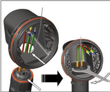
**13.** Take out thermostat. Mount junction box base on expediter. Make sure to align slots to properly orient junction box base. Tighten nut with Terminator-LN-Tool. If mounting horizontally, threaded gland holes must face downward.
