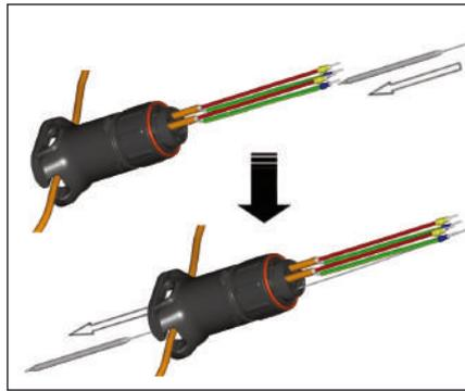
8. Route thermostat bulb through nut and expediter opening in junction box base. If necessary, apply lubricant (user supplied) to end of thermostat bulb. Slide through conical grommet hole. Push excess capillary tube through expediter.
