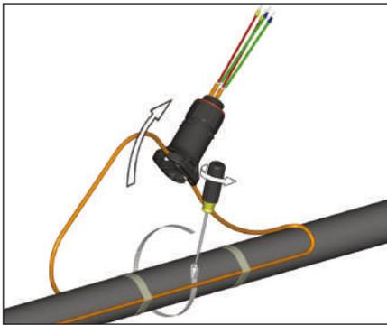
7. Remove expediter from pipe by removing pipe band.
