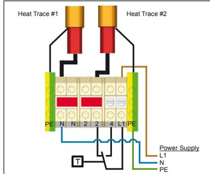
Thermostat Connection (2 Heating Cables)
