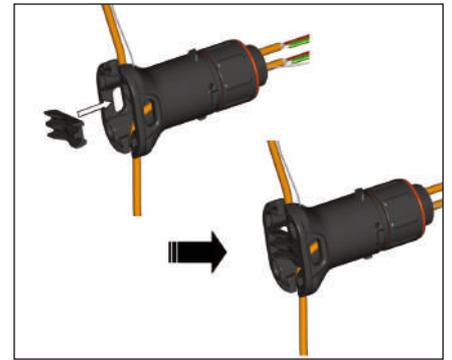
9. Insert banding guide and snap into place.
