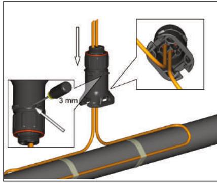
2. Insert cable into expediter. If mounted on bottom or side of pipe, punch out weep hole.
